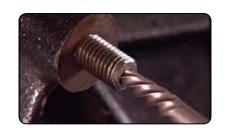
Damaged bolt remove / Screw extractor Page 8-20 ~8-23
