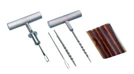
For steel belted redial tire. T-handle disclosed tire repair tool is for inserting plugging material typically in the form of rubber coated strands, into a tire puncture. The plugging material is threaded into the open eye of a needle forming a part of the tool and inserted into the puncture. The inserting motion is limited by a stop free to rotate on the needle's shank so that the ends of the strand are not drawn into the puncture and the stop also limits the withdrawal of the needle.
