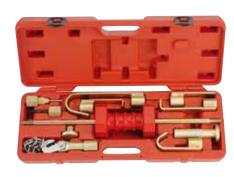
For those hard to reach places on unit-sized body reconstruction, when working on fenders, rocker panels, door edges, bumper ends, aligning doors, hoods, trunks etc. hammers both ways without reversing. Solid 5/8" steel slide shaft, pipe end nose adapter is machined and plated.
