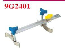
• It's designed to lock twin camshafts to timing marks during timing belt replacement. Fit onto sprockets and extend to lock in to sprocket teeth adjustable arms.
