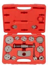
• For rotating pistons back into the caliper to provide clearance for new pads. Include 11 adaptors (available individually) for use in both 2 and 4-wheel rear disc brake assemblies of most domestic and import cars. The tool may be used "on" and "off" the car.
