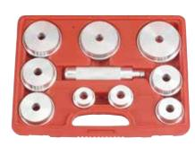
Makes it easier to insert wheel bearing race and seals without damage to race and axle housing. The set includes 9 disc sizes to fit most standard wheel bearing. Turn discs over to drive seals.
