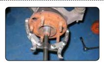
Puller tool (bearing / gear separator)
