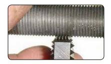
Threaded repair / Nut cracker tool Page 8-23 ~8-27
